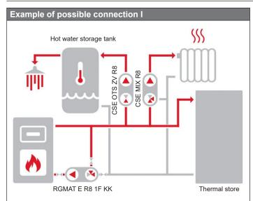
The diagram shows a typical connection of a solid fuel boiler, thermal store and heating circuit (with the recommended CSE MIX R8 pump station – not included in supply). If the boiler is used also for hot water heating, it is recommended to install a CSE OTS ZV R8 pump station (not included in supply).
