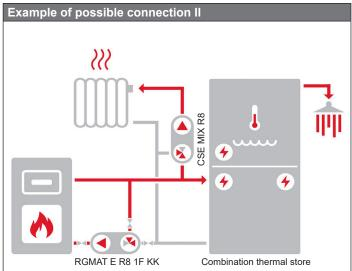
The diagram shows a typical connection of a solid fuel boiler, combination thermal store and a heating circuit (with the recommended CSE MIX R8 pump station – not included in supply).
