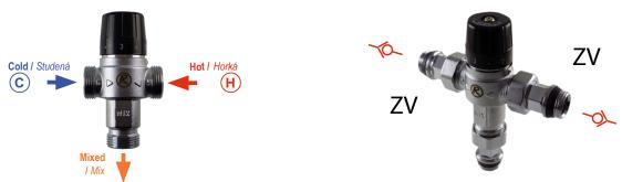
Moreover, the valve features an anti-scalding function. In case of cold water supply breakdown, the hot water supply is interrupted as well. This safety function works from 10 K temperature difference between the incoming DHW and mixed hot water. Its functionality can be checked by closing cold water supply; the flow through the thermostatic valve should drop to zero very fast.
