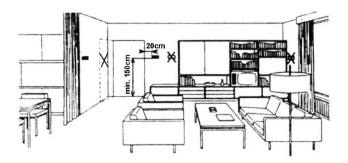
This thermostat is intended for indoor use only. It should be mounted on an inner wall, about 150cm above the floor, located where it can easily sense an air sample that is consistent with room temperatures.
