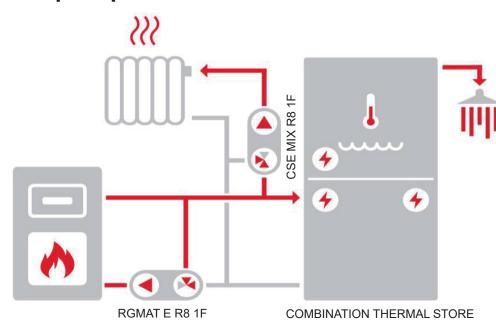
The diagram shows a typical connection of a solid fuel boiler, combination thermal store and heating circuit (with the recommended CSE MIX R8 1F pump station – not included in supply).
