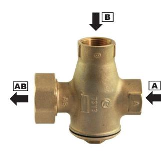
The TSV3B load valve is fitted with an integrated thermostatic insert that will close the A inlet (from a heating system), if the return water temperature to the boiler (AB outlet) is lower than the opening one. As soon as the opening temperature is reached, the thermostat starts opening the A inlet slowly and mixing the cold return water with the hot water from the B inlet (boiler flow) with the aim to reach the opening temperature (AB outlet) in the return pipe.
