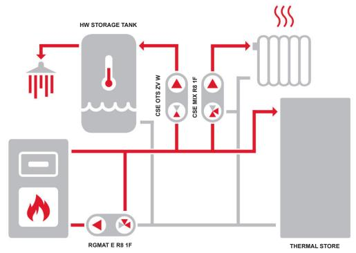
The diagram shows a typical connection of a solid fuel boiler, thermal store and heating circuit (with the recommended CSE MIX R8 1F pump station – not included in supply). If the boiler is used also for hot water heating, it is recommended to install a CSE OTS ZV W pump station (not included in supply).
