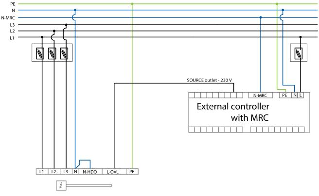
El. heating element - accumulation tank
