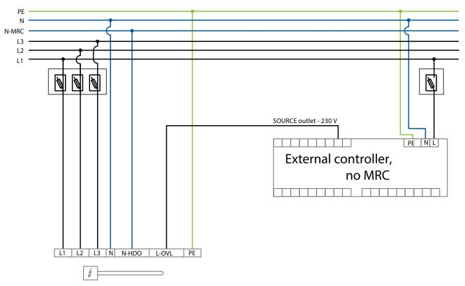
El. heating element - accumulation tank
