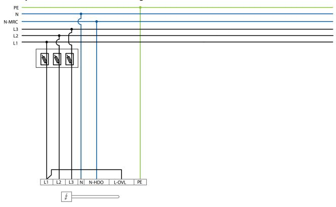
El. heating element - accumulation tank
