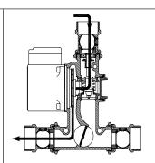
As soon as the nominal temperature is reached, the thermostatic valve starts opening the return line so that a constant nominal temperature is reached for return water by mixing it with water circulating via bypass.
