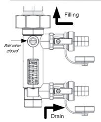
(1) - Filling the installation: Remove the plugs from the side valves and connect the hose unions. Close the ball valve and open the side filling valve and draining valve.
