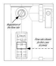
(3) - Regulate the flow rate using the regulation rod until the right flow rate is shown.
