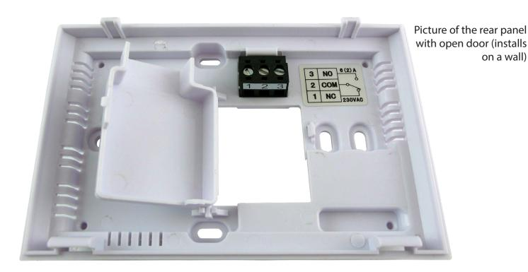
**Heating:** connect the two connecting cables of the controlled device to terminals No. 3 (NO – normally open) and No. 2 (COM).
