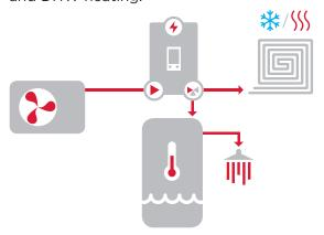
RegulusBox combined with a heat pump and a combination thermal store in systems for space and DHW heating.
